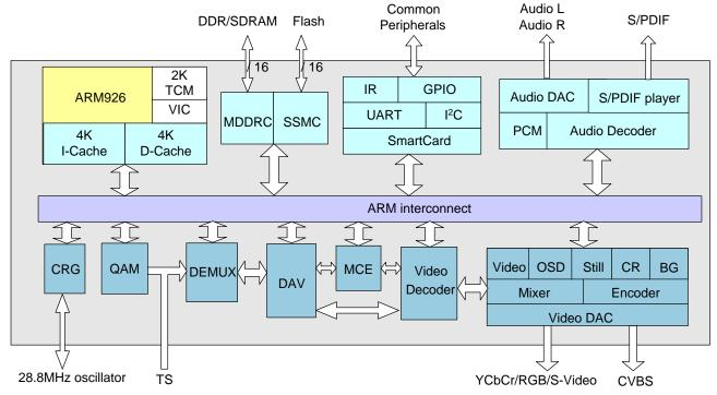
The Hi3110Q is a SoC chip that integrates the Quadrature Amplitude Modulation (QAM) demodulation and MPEG-2 source decoding functions. It offers a highly cost-effective DVB-C system solution and an excellent integrated machine solution in the industry.
