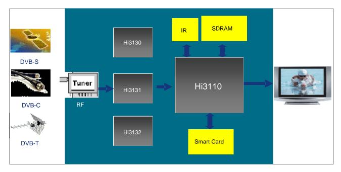
The Hi3110Q is a high-performance SoC chip that provides the MPEG-2 source decoding functions and integrates a QAM demodulator. It offers a low-cost cable digital TV set-top box solution.
